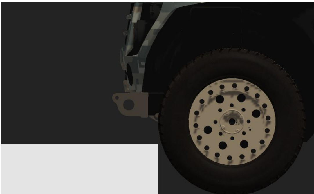
Figure 15: Vehicle crossing 12-inch step
