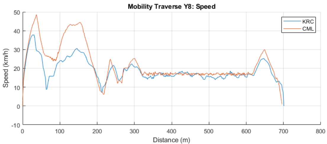
Figure 26 Simulated and test speeds for traverse section Y8
